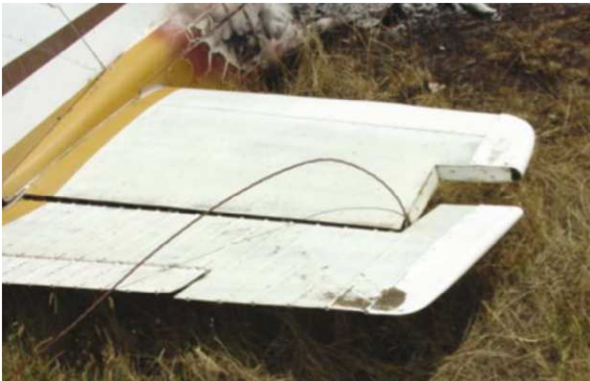
Tragedy on Christmas morning. Section of the struck powerline caught in the horizontal stabiliser
