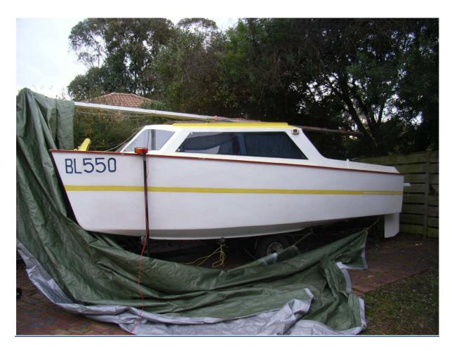
Having given up flying after a slight stroke I have resurrected the boat I built about 24 years ago. It is a "Jarcat" cruising catamaran. 4.8 metres long with 2 sails (self-furling jib and main), 'metho' stove, chemical toilet and electric shower; also powered by a 9.9hp Mercury Sail Power outboard motor. 10 knots flat out but up to 20 knots under sail.
