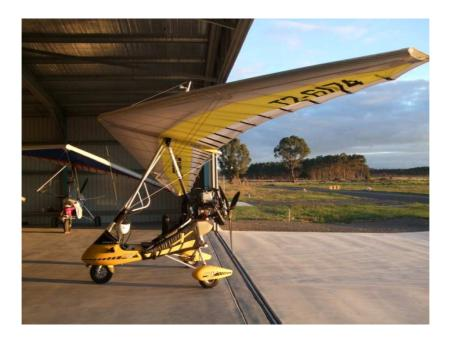
Airborne Edge X Classic, Rotax oil injected 582 with Streak 2B wing, 2005 build.
