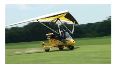
The Reflex wings now come in 4 sizes – so the triker has a good range to select from. There is the Reflex 11, 12, 13 and 15. The number refers to the size or square metres of the wing. The electric inflight adjustable speed trim gives effortless cruise up to 87 knots and as low as 55 knots (in the case of the Reflex 11 wing). Also all Reflex wings are quick fold wings – meaning that they can be folded while still on the trike to be quickly put away in a small space in a hangar.
